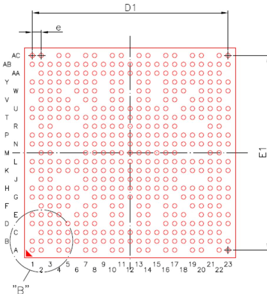
Fig. 2-4 RK3368H TFBGA453 Package Bottom View
