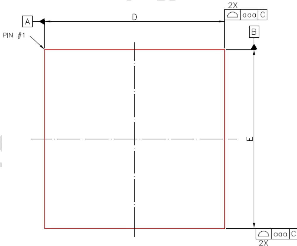
Fig. 2-1 RK3368H TFBGA453 Package Top View
