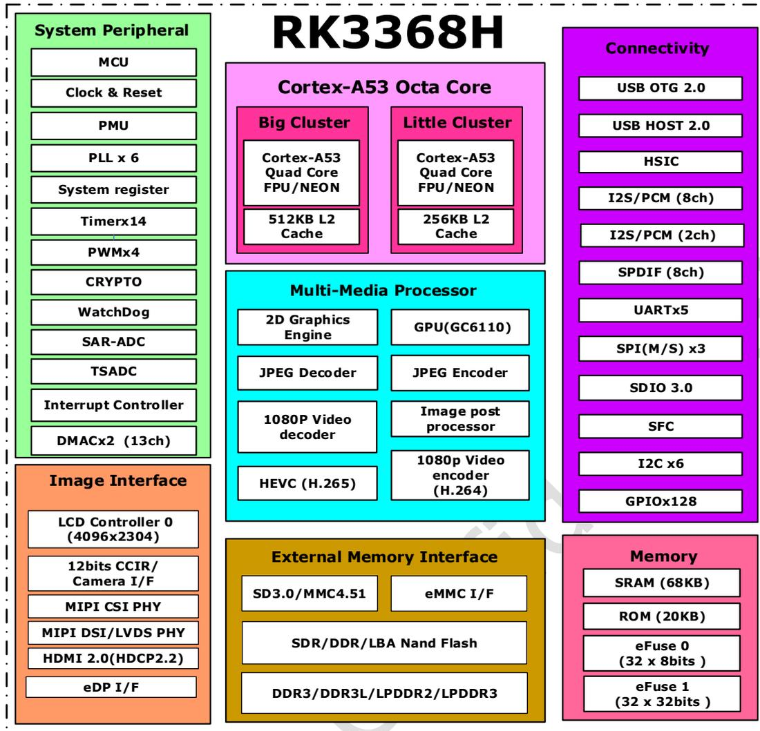
Fig. 1-1 RK3368H Block Diagram
