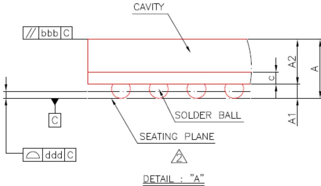
Fig. 2-2 RK3368H TFBGA453 Package Side View
