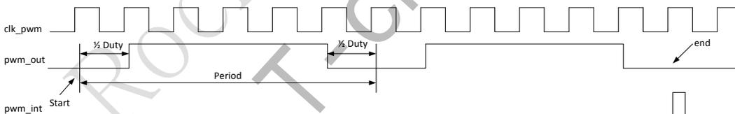
Fig. 51-5 PWM Center-aligned Output Mode
