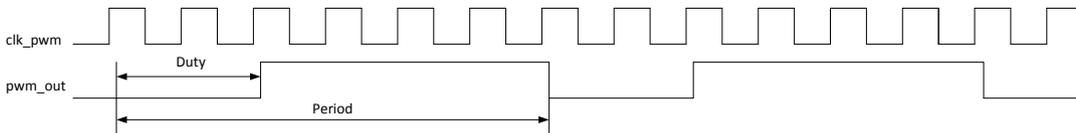
Fig. 51-3 PWM Left-aligned Output Mode
