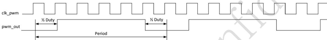
Fig. 51-4 PWM Center-aligned Output Mode
