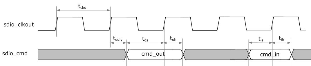
Fig.4-29 SDIO CMD Interface Timing
