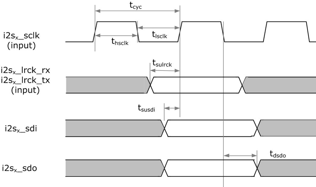
Fig. 4-28 Slave mode timing diagram
