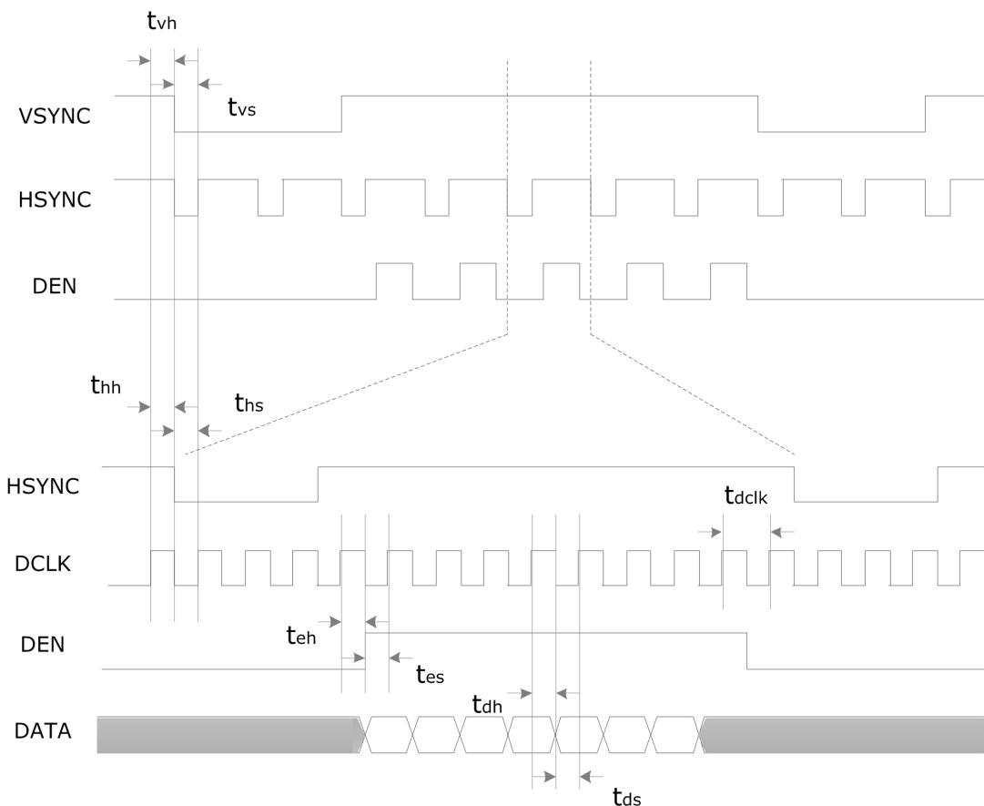
Fig. 4-22 LCDC RGB interface timing (SDR)
