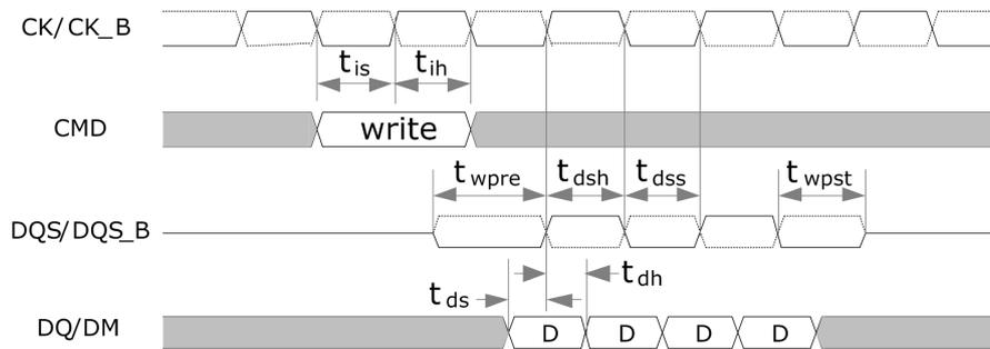
Fig. 4-3 LPDDR2 burst write operation: WL=1, BL=4
