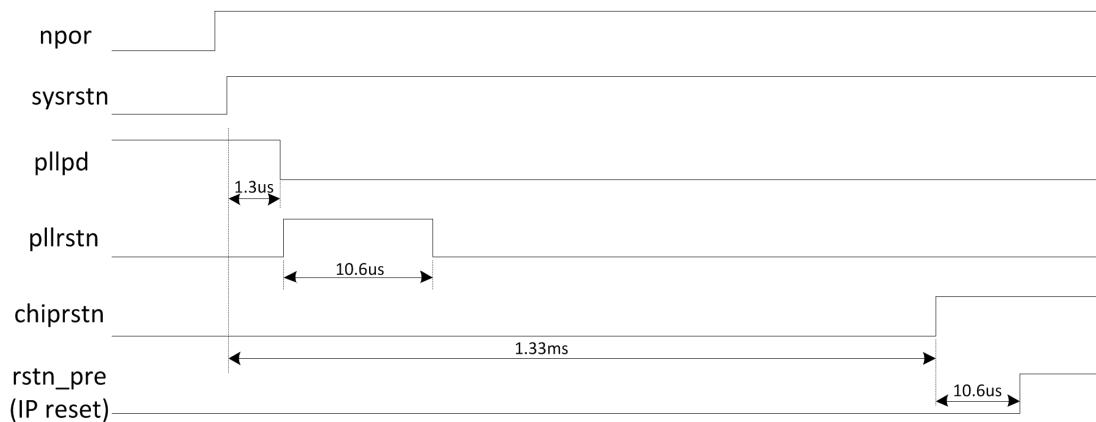
Fig. 5-4 RK3188T reset signals sequence
