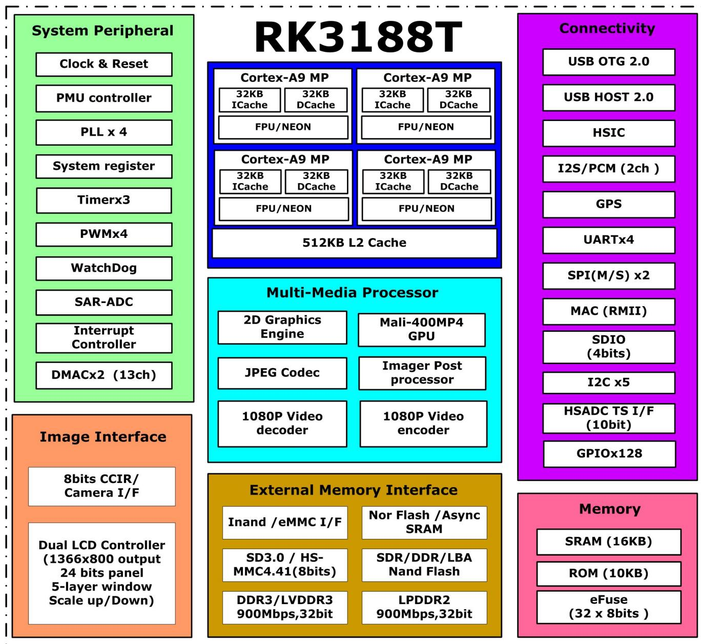
Fig. 1-1 RK3188T Block Diagram
