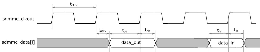
Fig. 4-21 SDMMC Data Interface Timing
