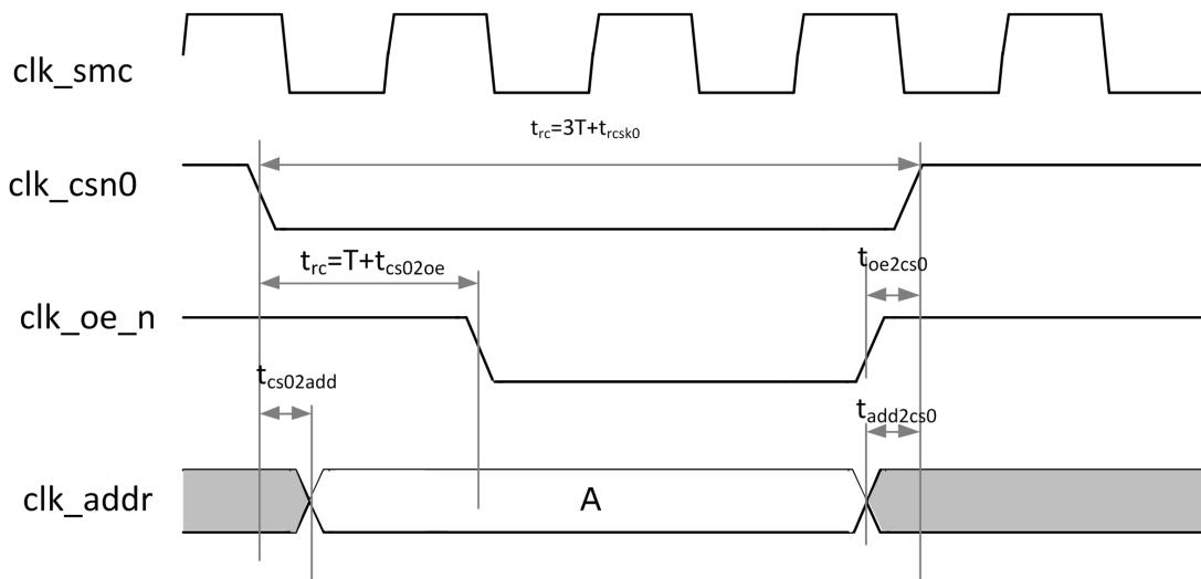
Fig. 4-5 SMC timing diagram of asynchronous read
