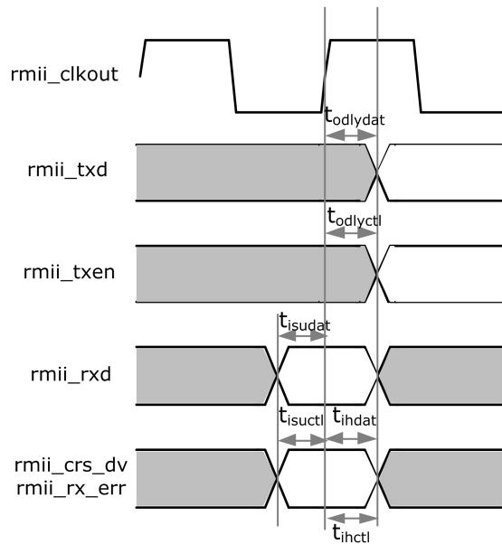
Fig. 4-32 RMII timing diagram
