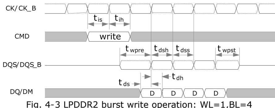
Fig. 4-3 LPDDR2 burst write operation: WL=1, BL=4
