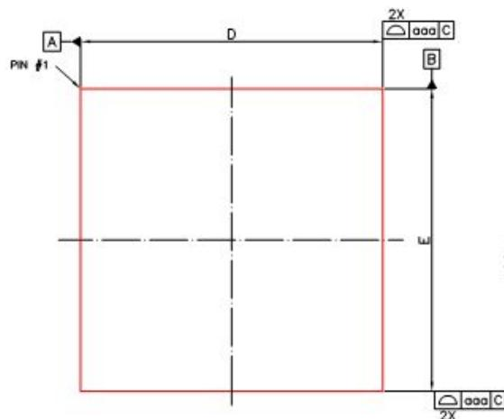
Fig. 2-1 RK3188T TFBGA453 Package Top View
