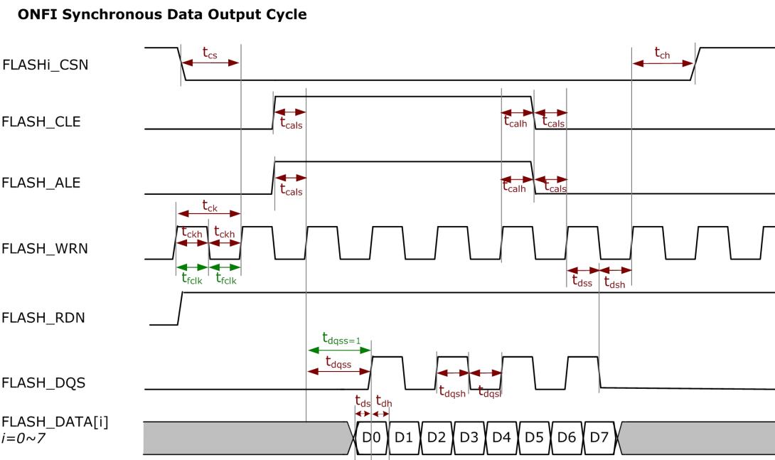
Fig. 4-12 NandC ONFI Syn Data Output Cycles
