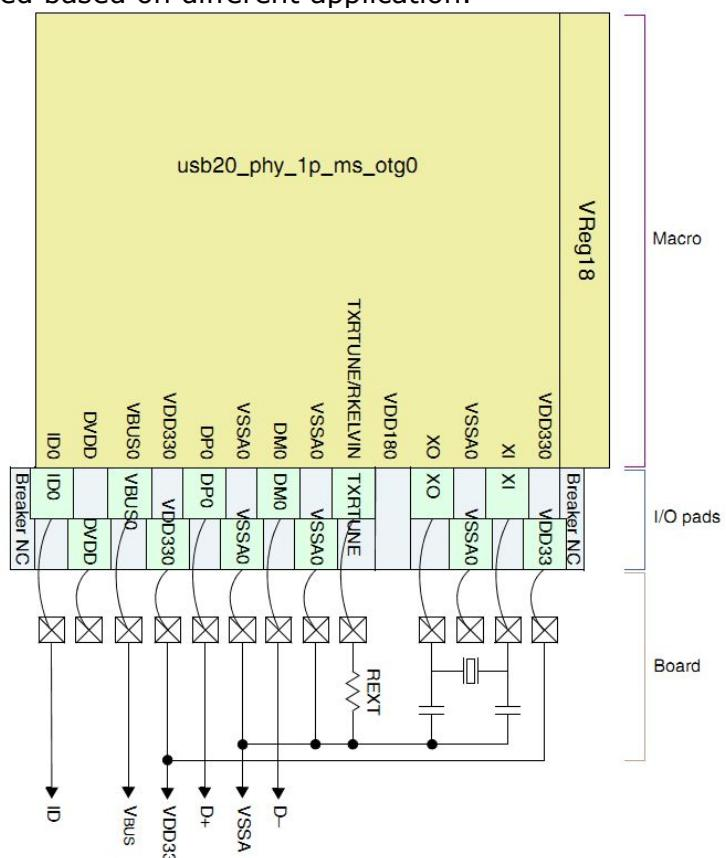
Fig. 5-3 RK3188T USB OTG/Host2.0 interface reference connection
