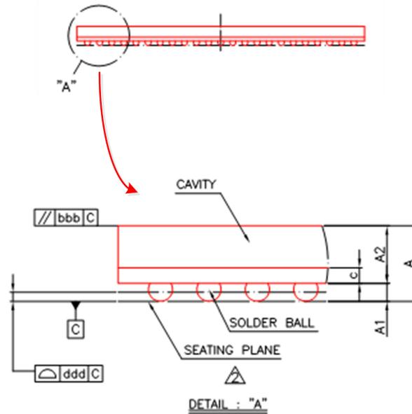
Fig. 2-2 RK3188T TFBGA453 Package Side View
