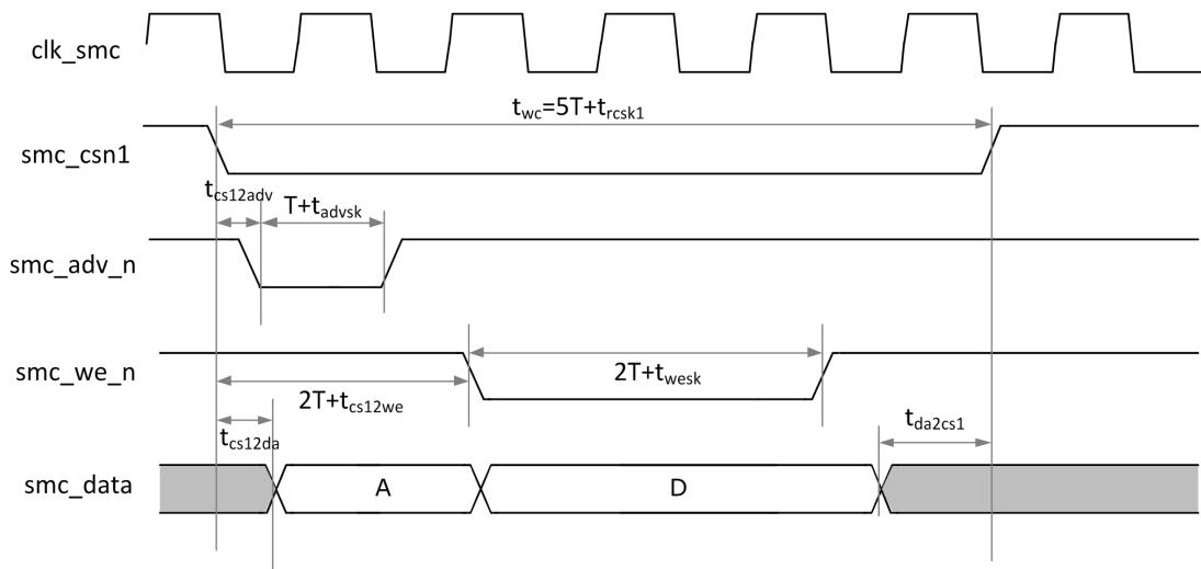
Fig. 4-6 Asynchronous Write Timing Diagram In Multiplexed Mode
