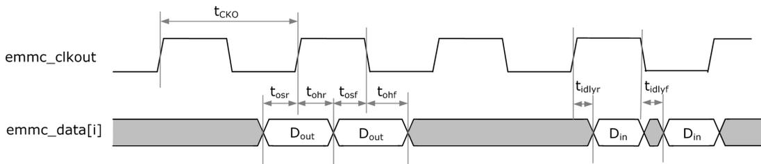
Fig.4-18 eMMC Data Interface Timing, DDR4 Mode
