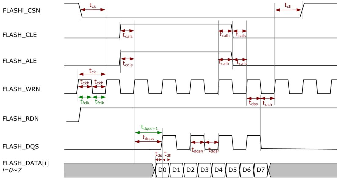
Fig. 4-12 NandC ONFI Syn Data Output Cycles
