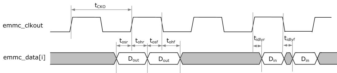
Fig.4-19 eMMC Data Interface Timing, DDR8 Mode
