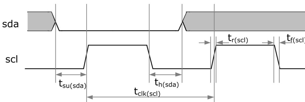
Fig. 4-36 I2C timing diagram
