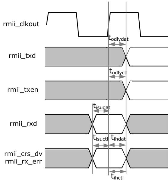
Fig. 4-32 RMII timing diagram
