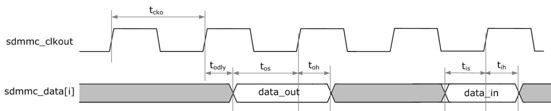
Fig. 4-21 SDMMC Data Interface Timing
