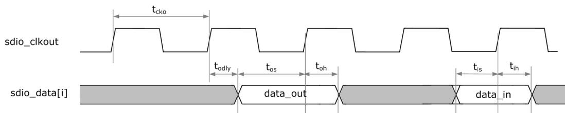
Fig. 4-30 SDIO Data Interface Timing
