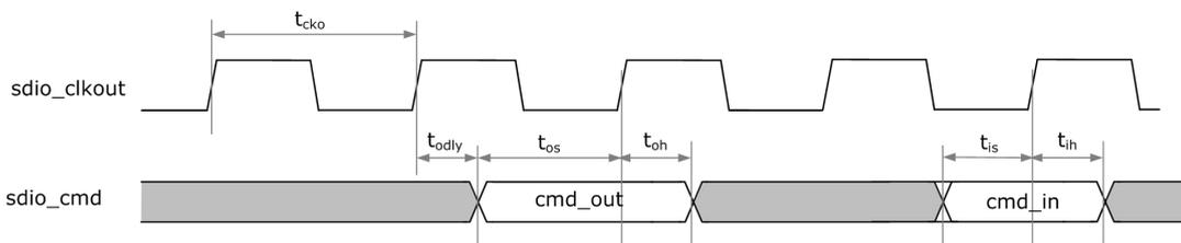
Fig.4-29 SDIO CMD Interface Timing
