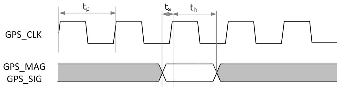
Fig. 4-26 RK3188T GPS timing waveform
