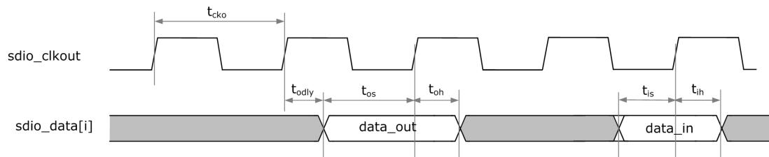
Fig. 4-30 SDIO Data Interface Timing
