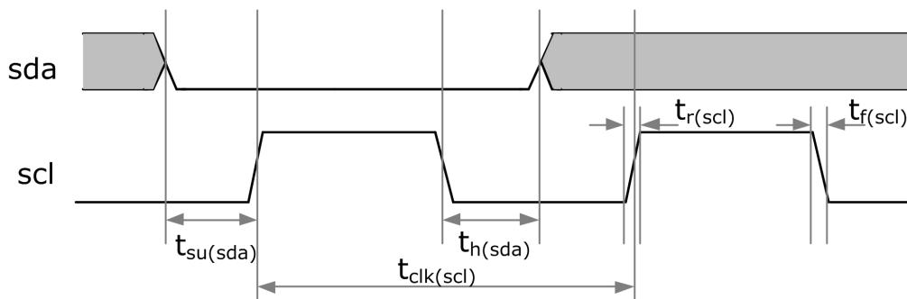
Fig. 4-36 I2C timing diagram
