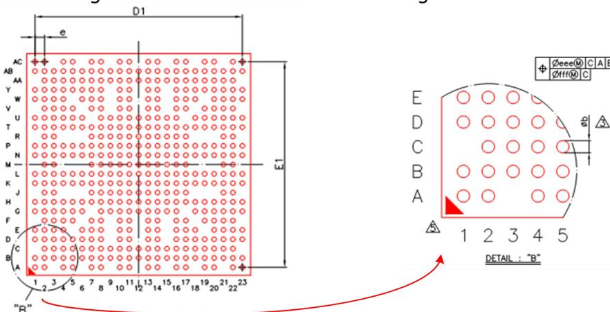
Fig. 2-3 RK3188T TFBGA453 Package Bottom View
