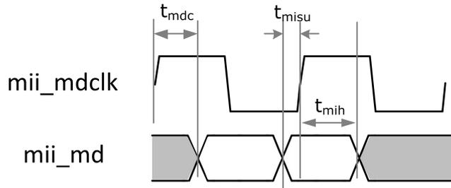
Fig. 4-31 Management timing diagram
