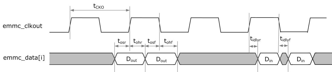
Fig.4-18 eMMC Data Interface Timing, DDR4 Mode
