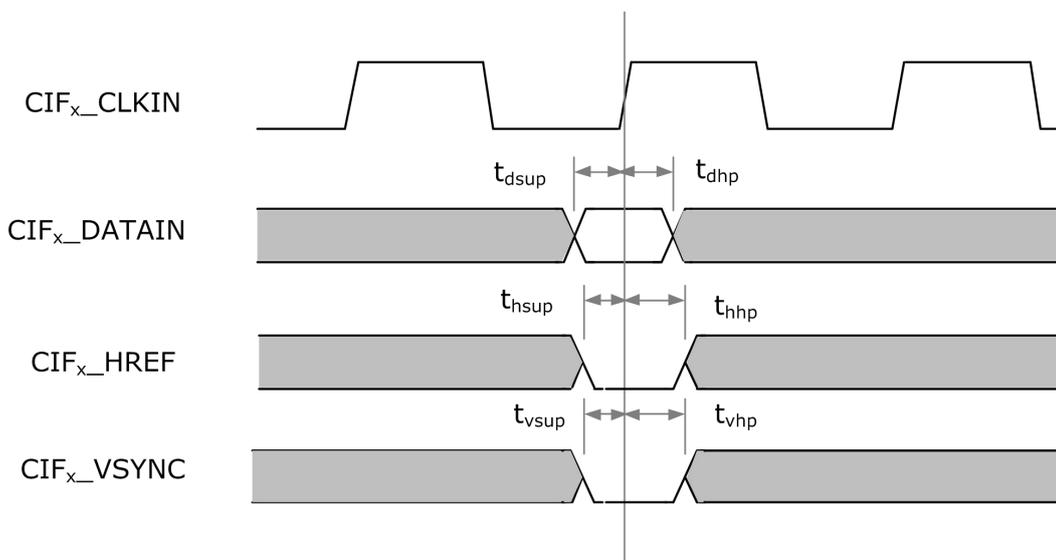
Fig. 4-25 CIF timing diagram
