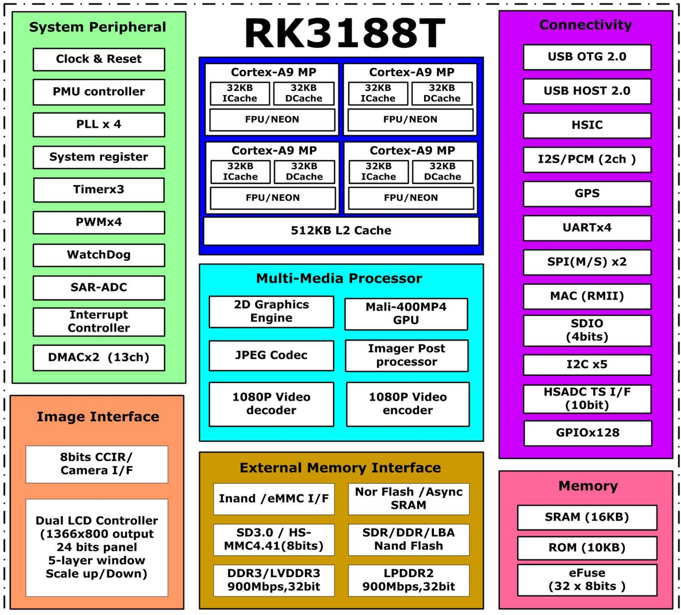
Fig. 1-1 RK3188T Block Diagram
