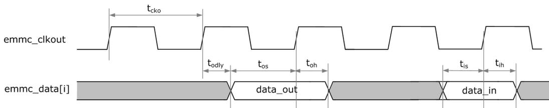
Fig.4-17 eMMC Data Interface Timing
