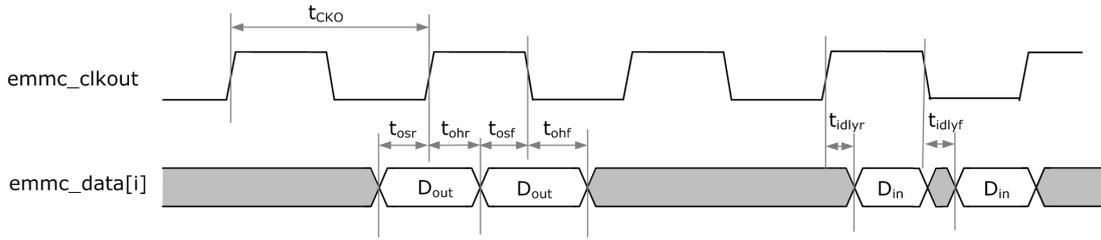
Fig.4-19 eMMC Data Interface Timing, DDR8 Mode
