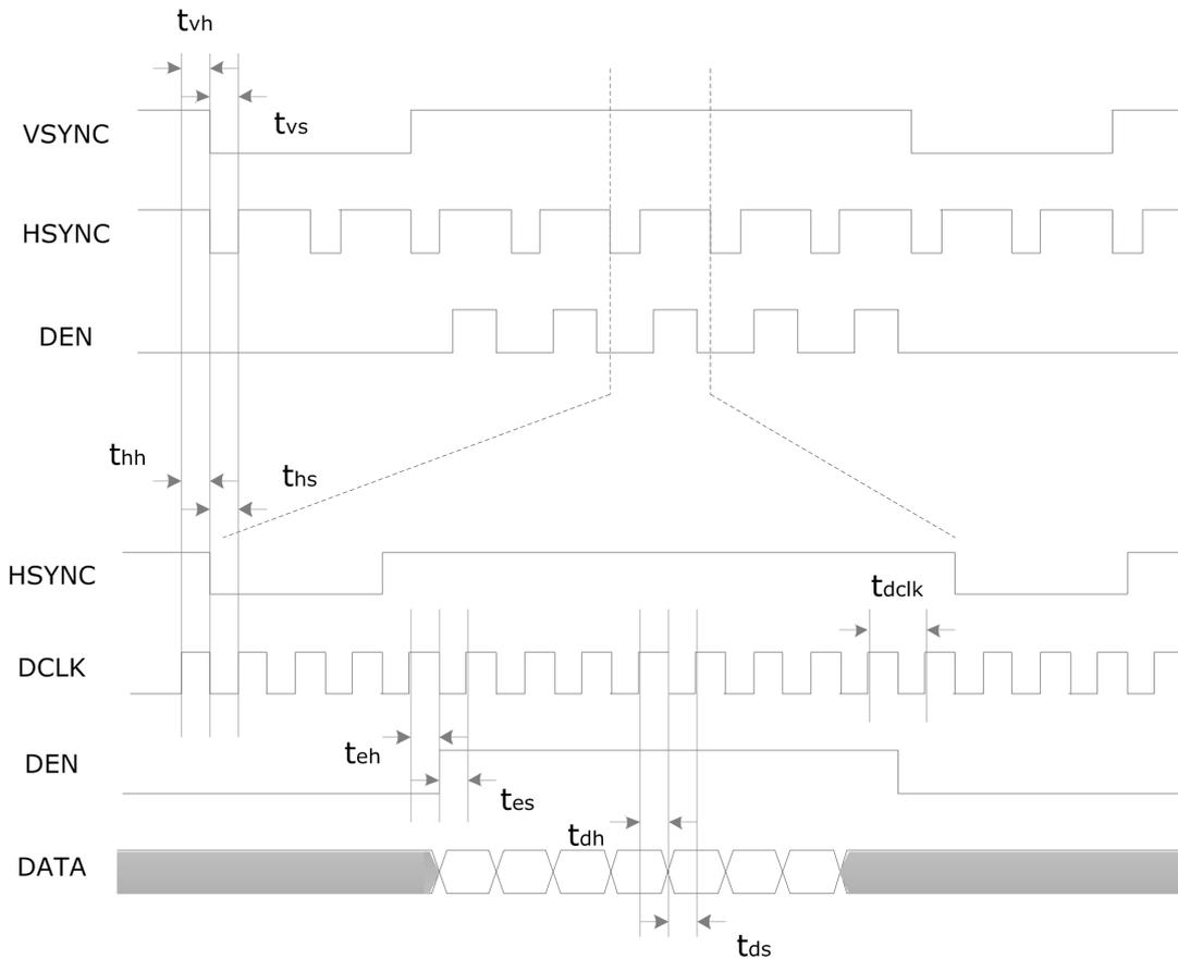
Fig. 4-22 LCDC RGB interface timing (SDR)
