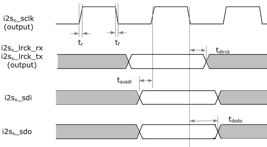
Fig. 4-27 Master mode timing diagram
