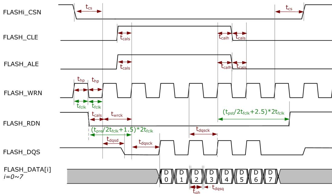
Fig. 4-11 NandC ONFI Synchronous Data Input Cycles
