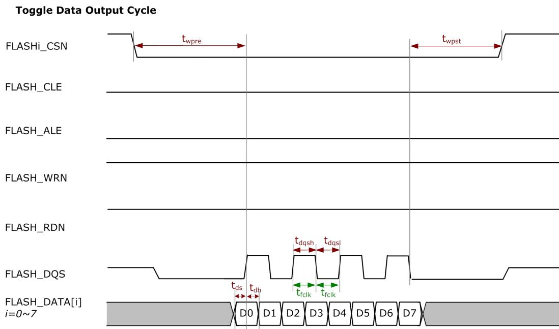
Fig. 4-15 NandC Toggle Data Output Cycles
