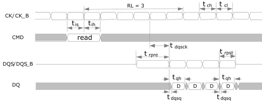
Fig. 4-4 LPDDR2 burst read operation: RL=3, BL=4
