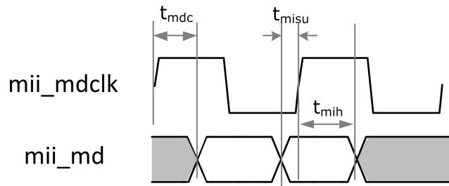
Fig. 4-31 Management timing diagram
