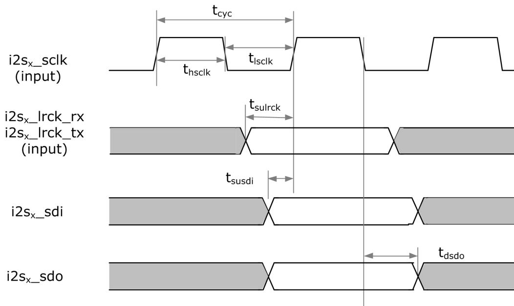
Fig. 4-28 Slave mode timing diagram
