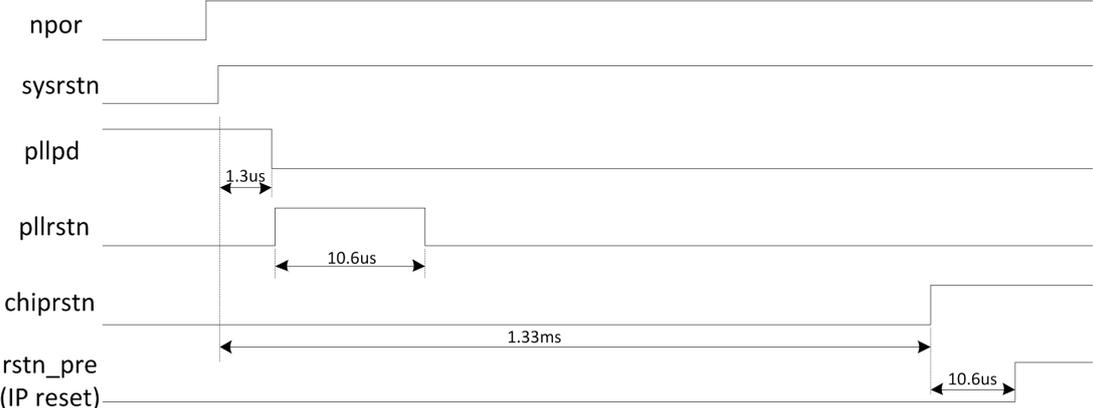
Fig. 5-4 RK3188T reset signals sequence
