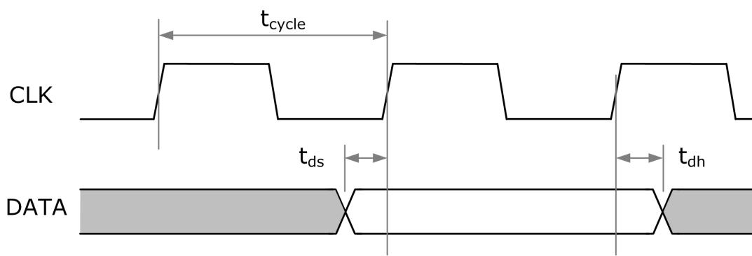
Fig. 4-33 HS-ADC Interface timing diagram
