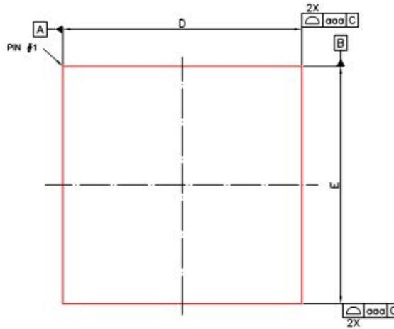
Fig. 2-1 RK3188T TFBGA453 Package Top View
