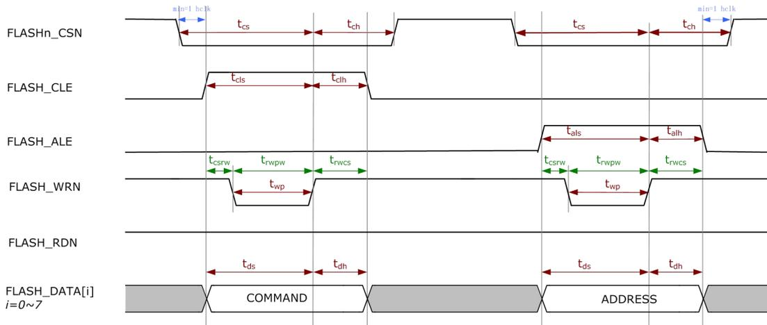
Fig. 4-13 NandC Toggle Address/Command Latch Cycle
