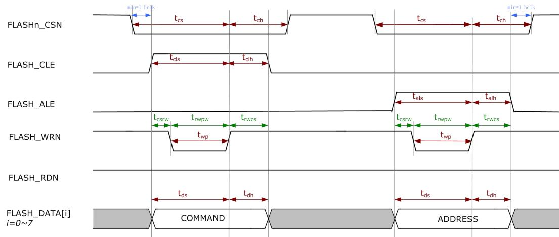
Fig. 4-13 NandC Toggle Address/Command Latch Cycle
