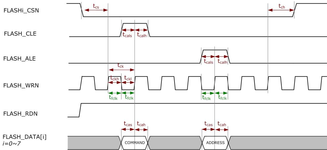
Fig. 4-10 NandC ONFI Syn Address/Command Latch Cycle
