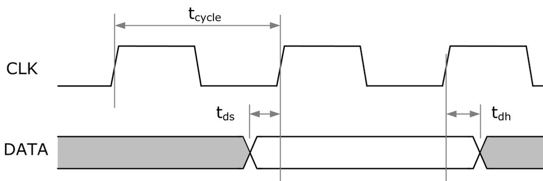
Fig. 4-33 HS-ADC Interface timing diagram
