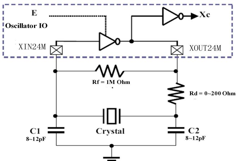
Fig. 5-1 External Reference Circuit for 24MHzOscillators
