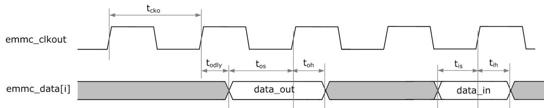
Fig.4-17 eMMC Data Interface Timing
