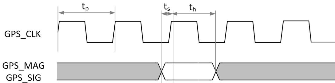
Fig. 4-26 RK3188T GPS timing waveform
