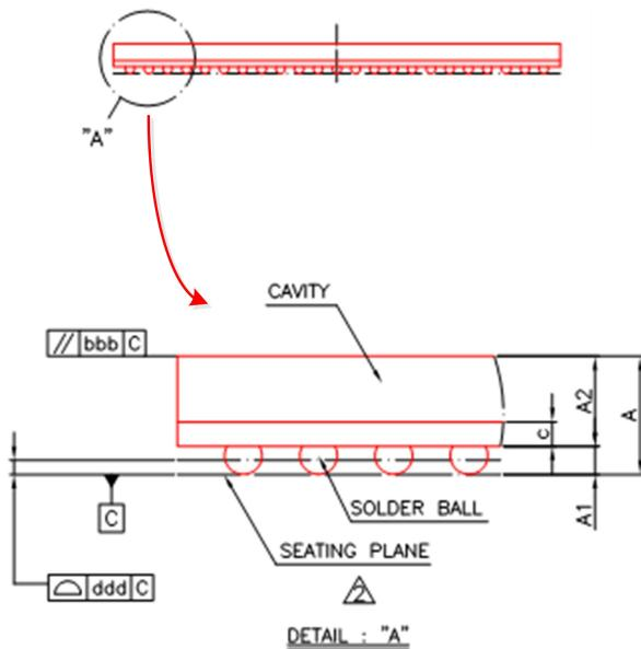
Fig. 2-2 RK3188T TFBGA453 Package Side View
