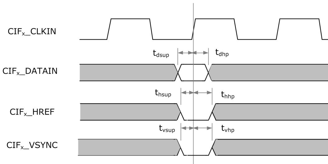
Fig. 4-25 CIF timing diagram
