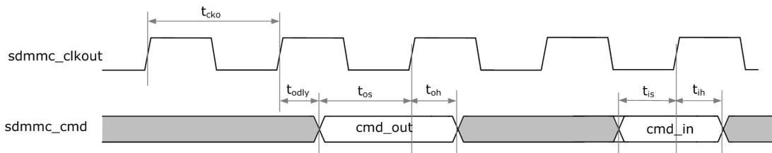
Fig. 4-20 SDMMC CMD Interface Timing
