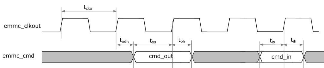
Fig.4-16 eMMC CMD Interface Timing
