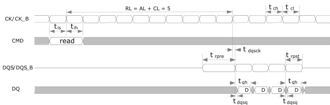
Fig. 4-2 DDR3 burst read operation:  $AL=0, CL=5$ , BC4
