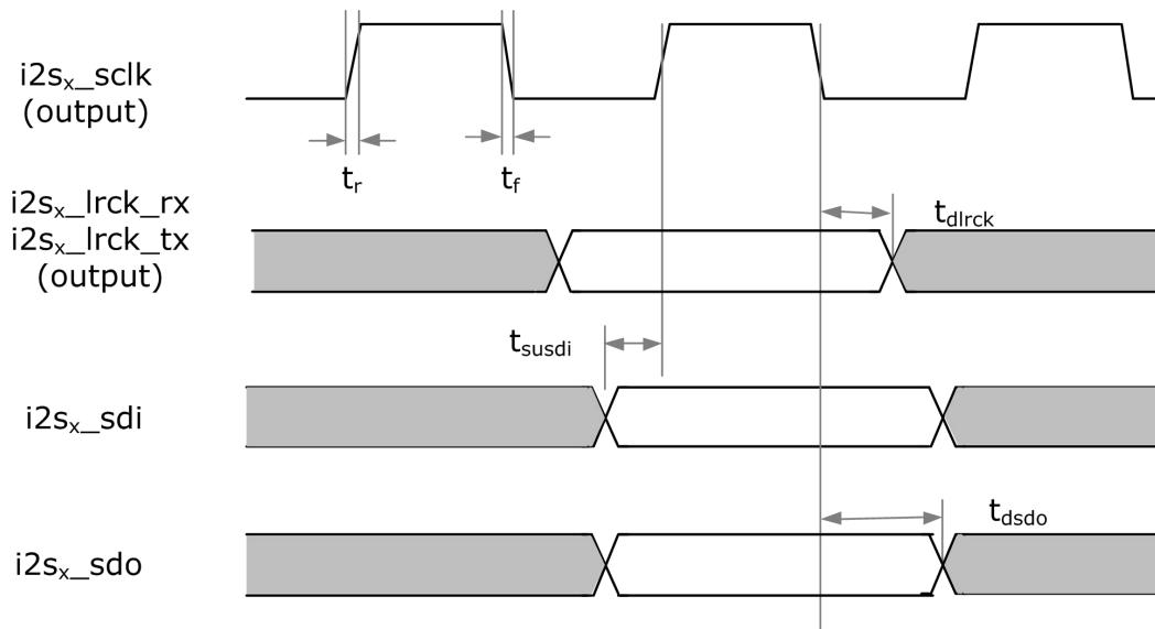
Fig. 4-27 Master mode timing diagram
