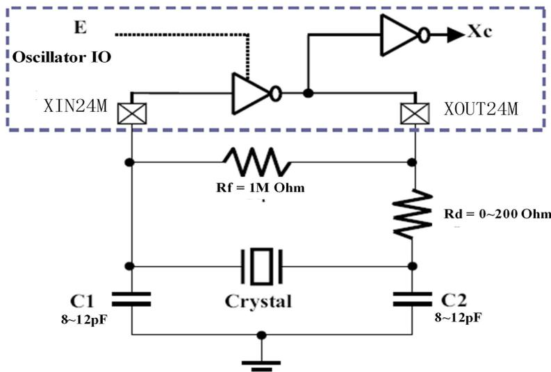
Fig. 5-1 External Reference Circuit for 24MHzOscillators
