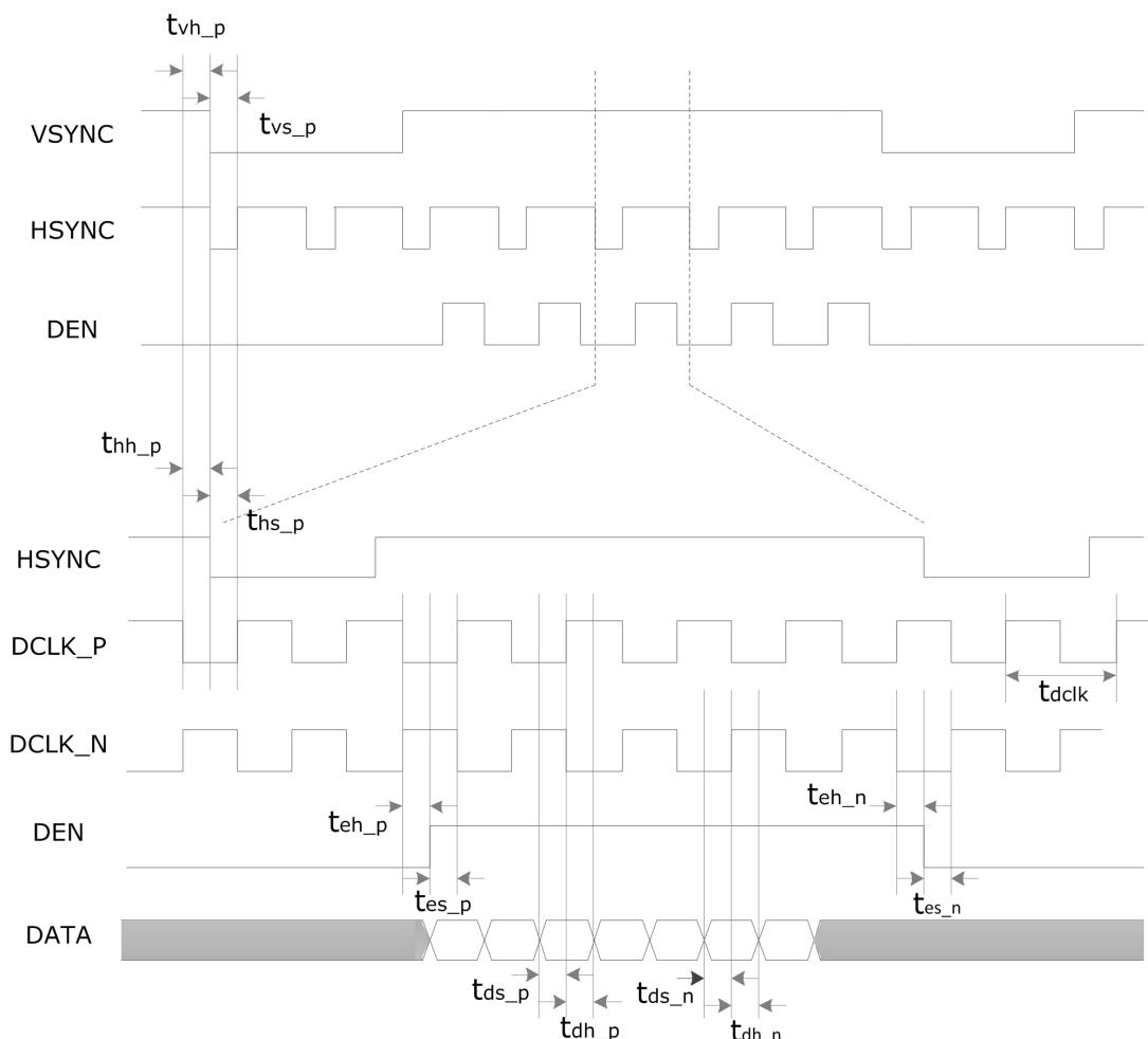
Fig. 4-23 LCDC RGB interface timing (DDR)
