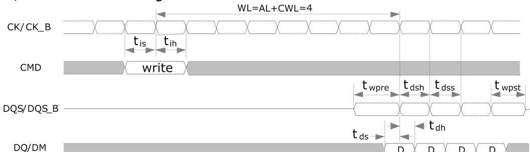
Fig. 4-1 DDR3 burst write operation:  $AL=0, CWL=4$ , BC4
